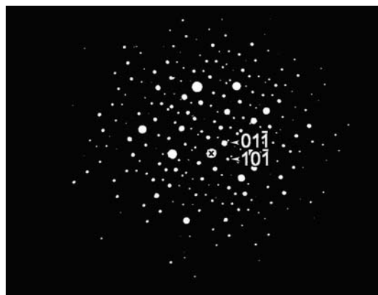
Fig. 3 Electron diffraction taken from zone axis [111] of \text{Mg}_{32}(\text{Al,Zn})_{49} phase. The transmitted beam is marked X. The pattern of the cubic \text{Mg}_{32}(\text{Al,Zn})_{49} precipitate (JCPDS19–29) is indexed
